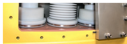
The bellows system is gastight.
